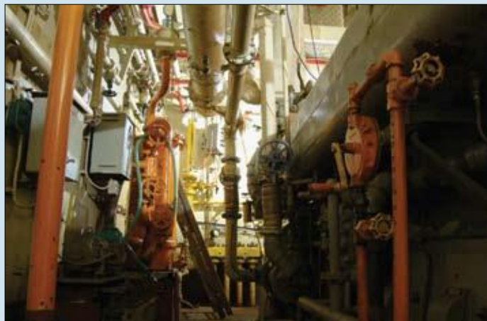
■ (Above left) The pilot house of the LV-112 as it appeared in 2010. (Above right) LV-112's main engine room in 2010. The main engine is on the right and yellow fuel, orange lube oil, and transfer/system valves are visible. — Photo courtesy of Tim May. (Left) The 7,000-pound main and 5,000-pound auxiliary mushroom anchors that held the LV-112 on station off Nantucket Shoals.
